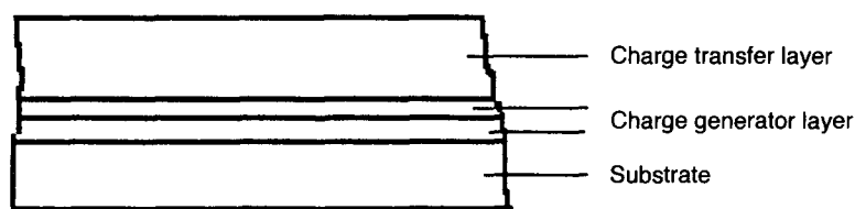
Fig. 1. Cross-section view of a photoreceptor device.
